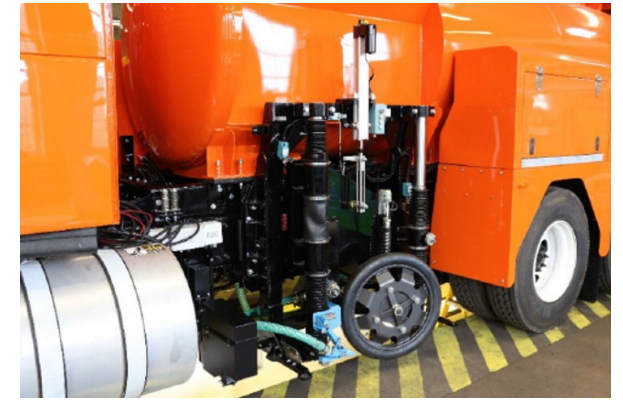
④ Sideway-force Coefficient Routine Investigation Machine ((SCRIM)
