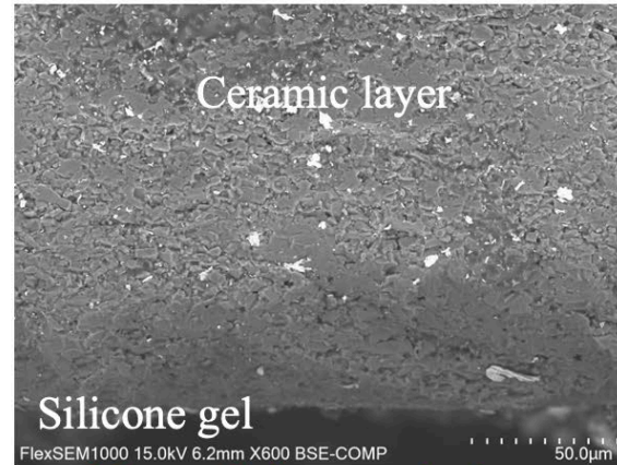
No crack in ceramic layer
